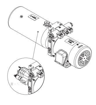
The W84A series power pack is designed for applications that need high pressure and larger flow,but use a low-power A.C. motor. Because the power pack uses a standard manifold(W800532), they will have the same functions as the W80A series power pack.
